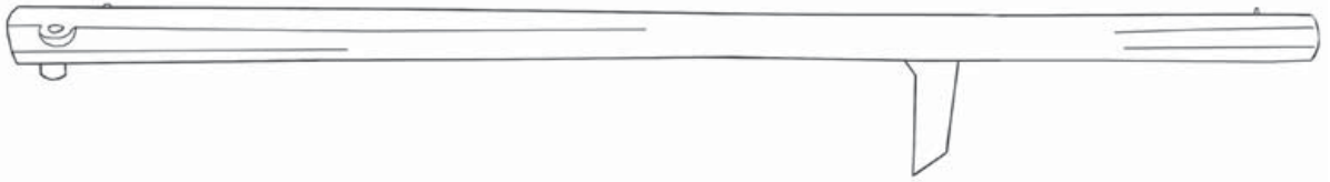
The barrel of a 16th-century 'hook-gun' or harquebus, known in Russian as a zatinnaya pishal or gakovnitsa . This example has a barrel nearly 4ft 6in long, of 0.9in calibre. (A.S. Sheps, after I. Ismailov)
